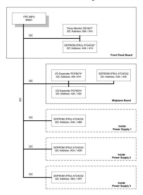
Figure 10-2: Devices Not Supporting Multimaster Mode
